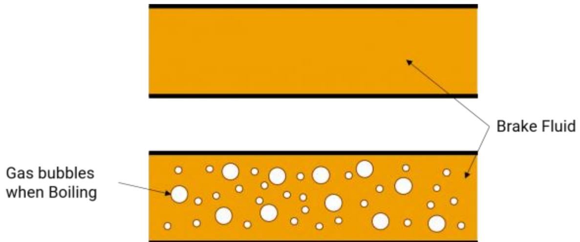
**Figure 3: Illustration of Gas in Brake Lines**
