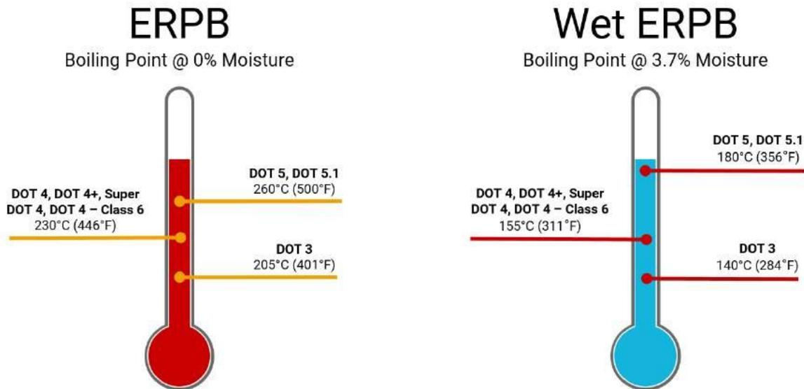
Boiling points for each fluid are shown in the illustration above. You'll notice that DOT 5, DOT 5.1 grades have the highest boiling points followed by DOT 4 (and its sub-grades) and then DOT 3.
